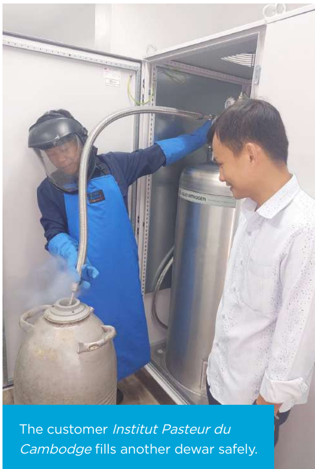
The CRYOGEN.65 filling an external dewar with liquid Nitrogen.
