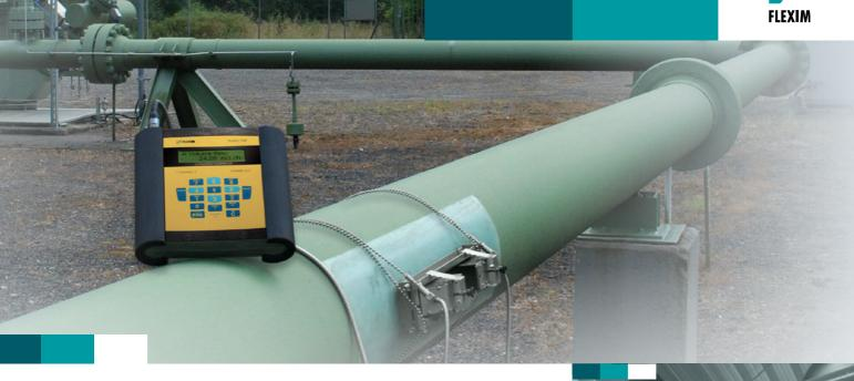
FLEXIM's range of FLUXUS® G60X portable gas flow meters not only covers virtually any gaseous medium, they also include all liquid flow metering capabilities of the FLUXUS® F60X series meter series making them a truly comprehensive tool.
